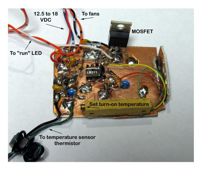
The thermistor is tucked inside the server PS near air outlet. Layer epoxy insulates it. Set potentiometer is multi-turn for ease of setting. Set turn-on temperature to suit. The LED is front panel mounted to show when fans are ON. Change the 1 M ohm resistor to vary the OFF – ON dead band (hysteresis). This revised circuit uses a low Rds MOSFET (3 milliohms) and is capable of switching 14 VDC of around 5-10 amps with no heat sink on the TO220 package. Much higher with heat sink.
