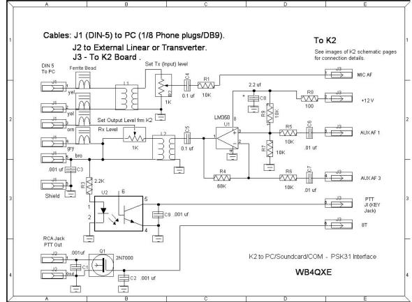
Above is the basic circuit. The left side (DIN5) is wired to a rear panel receptacle. On the right are the signals to and from the K2. Connectors (0.1" SIP) were used on the I/O board or on the K2 to ease removal and service. Female connectors, complete with shielded cable were scrounged from an antique VCR. Details of the "tap" points for the K2 are covered later.
