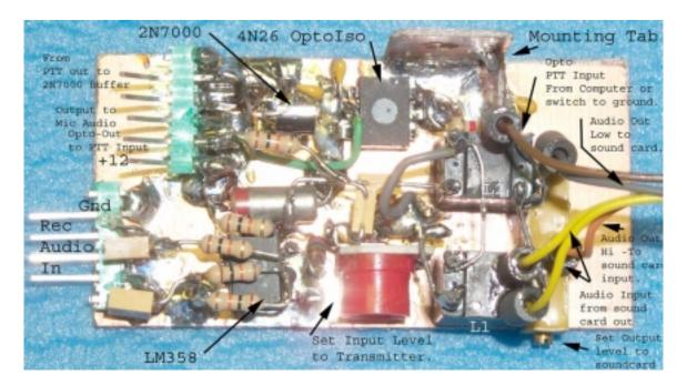
Here is a picture of the finished interface, before it was installed in the K2.
