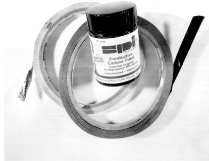
The double face tape, made conductive with carbon, is not an excellent conductor, but is quite sufficient for SEM work. Two faced tape and carbon "paint" are used "glue" specimens to a stub. Similar tapes and paints are available using other conducting materials such as silver, but carbon is cheaper and works well for most applications.
